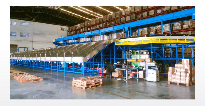
The first of its kind in the country with the capability to auto sort based on locations and route level for parcel up to 30kgs and 80cm in length. The system is being deployed at the 55,000 sq.ft eFMX e-Commerce shipment sorting center in Shah Alam and it is capable to sort up to 80,000 documents and parcels overnight within this facility.
